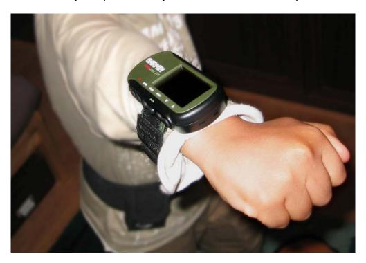
Figure 2 The Garmin Foretrex 201 GPS monitor
